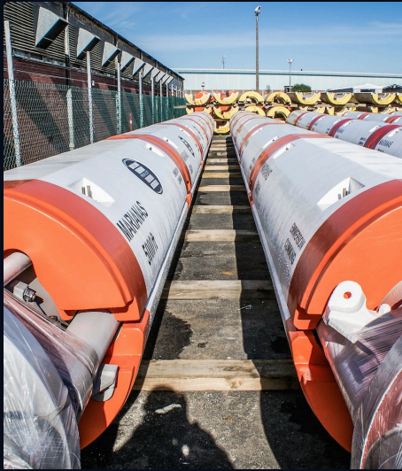
01 Riser joints dressed with buoyancy
